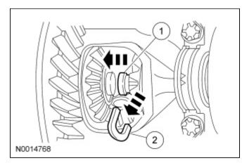
7. NOTICE: Do not damage the axle shaft oil seal.
