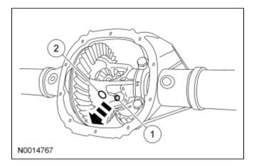
6. *NOTICE:* Do not damage the rubber O-ring in the axle shaft grooves.
