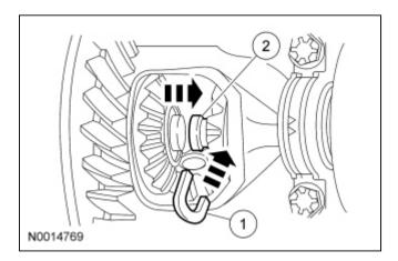
4. Install the differential pinion shaft.
