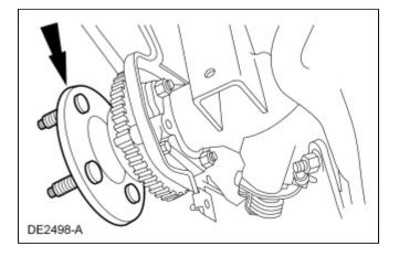
3. NOTICE: Do not damage the rubber O-ring in the U-washer groove.
